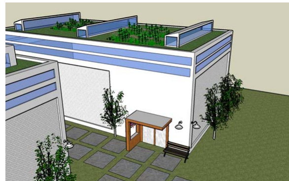
Green roofs reduce demand on stormwater management system and decrease heating and cooling costs by serving as additional insulation in the winter and deflecting radiant heat in the summer. Prepared for the City of Millville by the 2008 University of Pennsylvania – Planning Problems Workshop.
